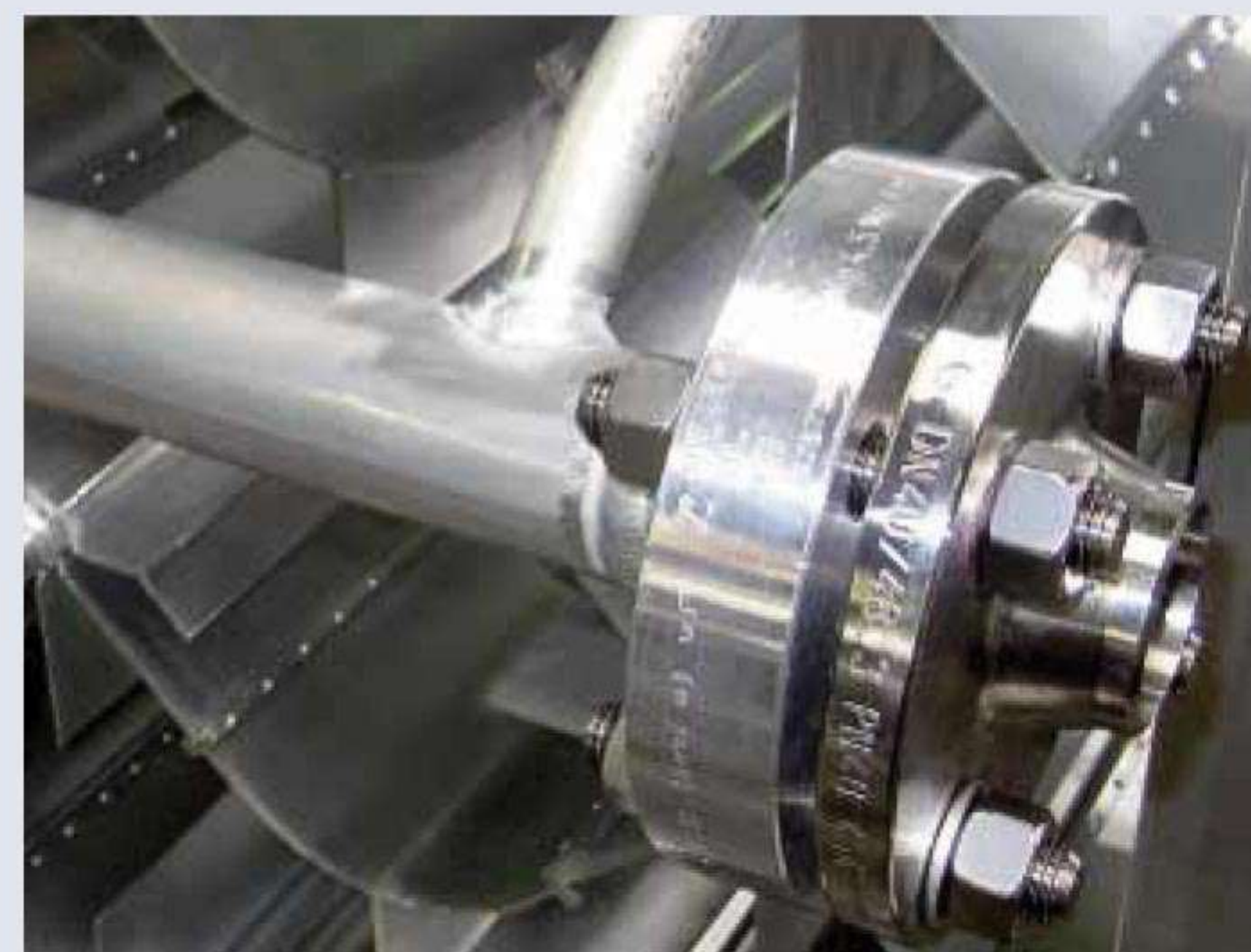
Flange - counter flange connection DN 40 / PN 40
