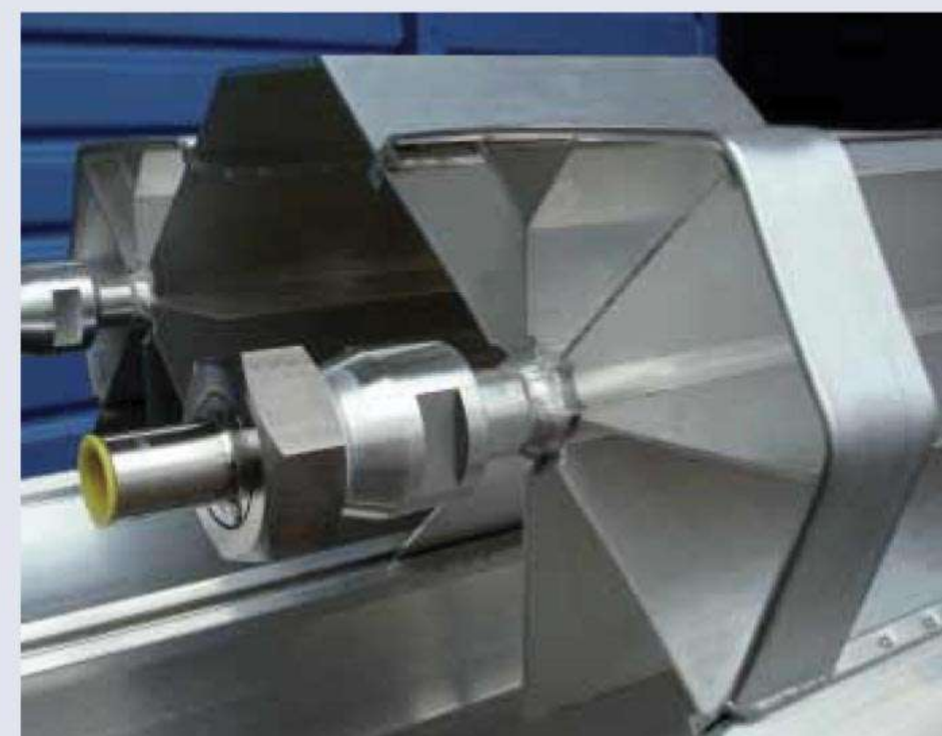
Screwed connection M40 x 2 as well as pipe connection. To protect the operating staff when connecting the intervening pipelines, HATCO evaporators are fitted with edge protection.
